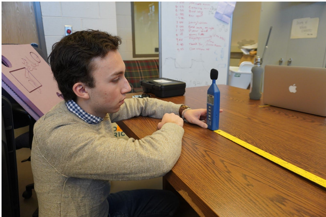
Figure 11: Phase one of PNC attenuation testing, capturing ambient data without the crate
